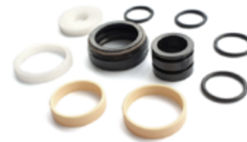
ROCKSHOX REVERB SERVICE KIT ND-130-001 INCLUDES 1 x ND Tuned RS Reverb Seal 1 x ND Tuned IFP + 4 x O-rings 1 x Upper + 1 x Lower Bushing 1 x Upper + 1 x Lower Foam Ring COMPATIBILITY RockShox Reverb seatpost A1/A2 B1/B2 MATERIAL NBR, POM, iglidur® J3
